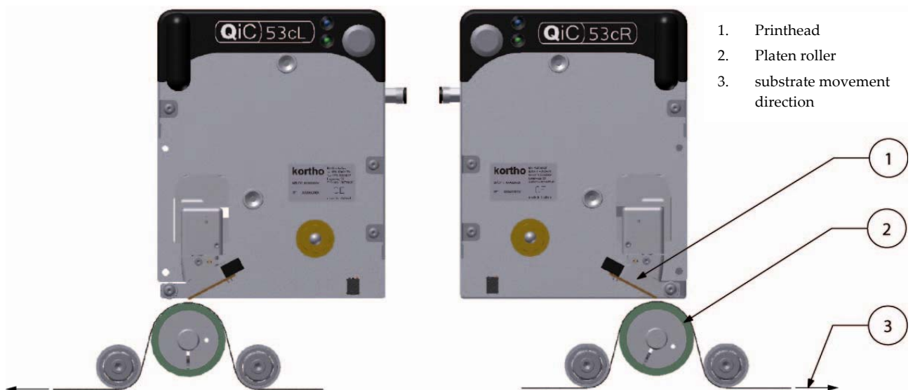
Fig. 2.6 Coding unit model selection
