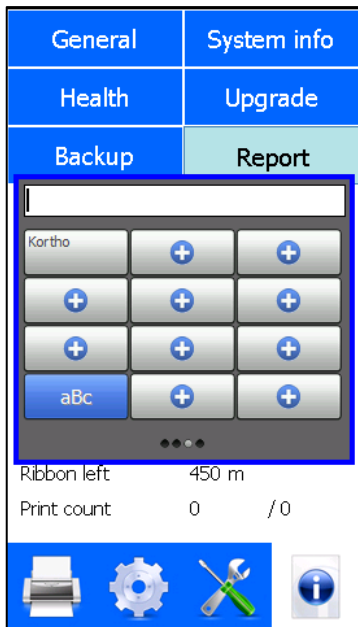
Fig. 3.9 Programming third keyboard screen buttons, entering text
