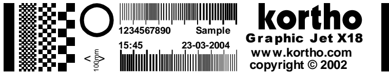
Fig. 7.11 Test label printed at correct speed setting (X18)
