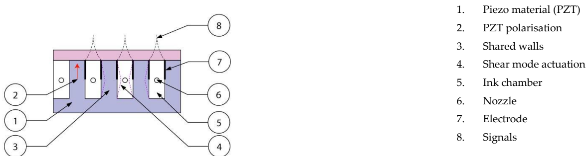
Fig. 3.1 Piezo printhead technology
