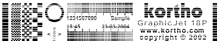
Fig. 9.5 Print result when nozzles are clogged with ink/dirt or blocked by air bubbles.
