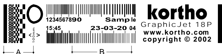
Fig. 9.8 Test image printed with variable product speed
