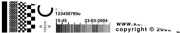
Fig. 9.4 Print result of air bubbles or reduced ink flow in ink system
