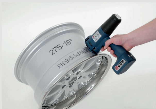
→ Aluminium printed with quick-drying ink (acetone); large spacing wheels.
