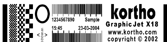
Fig. 9.43 Test image printed too fast, length < 100 mm (X72 <175mm)
