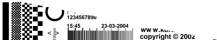
Fig. 9.41 Print result of air bubbles in the ink or reduced ink flow
