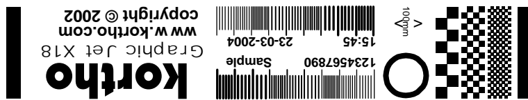
Fig. 7.14 Test label printed upside-down
