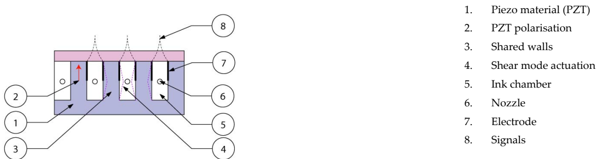
Fig. 3.1 Piezo printhead technology
