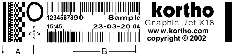
Fig. 9.45 Test image printed with variable product speed
