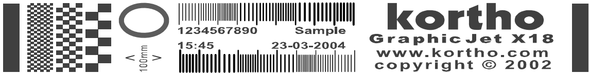
Fig. 9.44 Test image printed too slow, length > 100 mm (X72 > 175mm)
