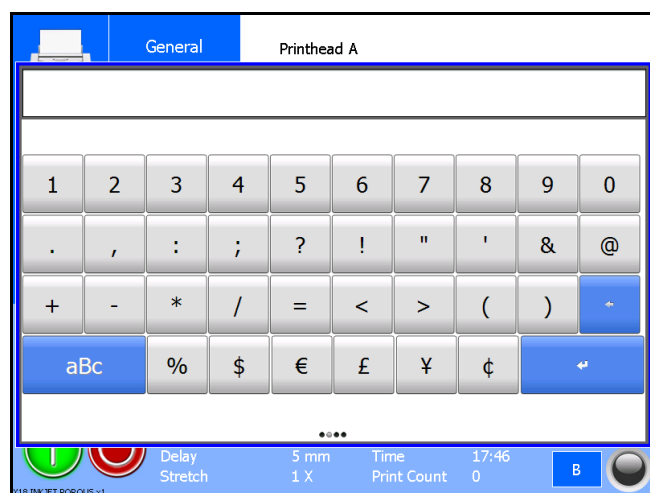
Fig. 3.7 Second keyboard screen, numeric and special characters
