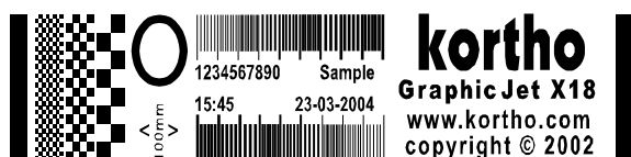
Fig. 9.43 Test image printed too fast, length < 100 mm (X72 < 175mm)
