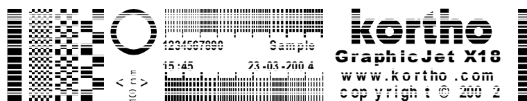
Fig. 9.42 Print result when nozzles are clogged with ink/dirt or blocked by air bubbles.
