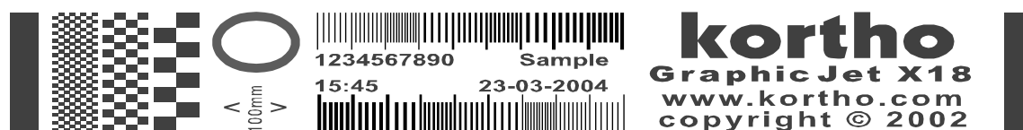
Fig. 9.44 Test image printed too slow, length > 100 mm (X72 > 175mm)
