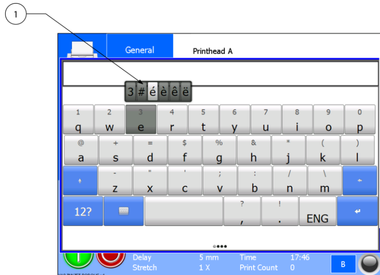
Fig. 3.6 First keyboard screen, alternative alphanumerics
