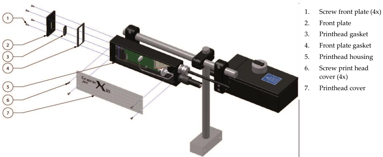
Fig. 10.1 Removing the printhead cover
