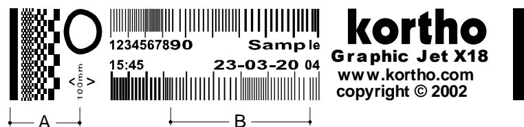
Fig. 9.45 Test image printed with variable product speed
