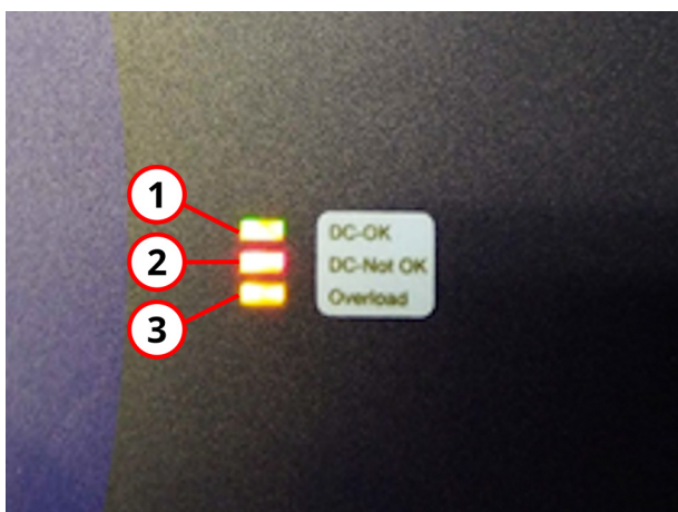
Figure 5-1: External Power LED Indication
