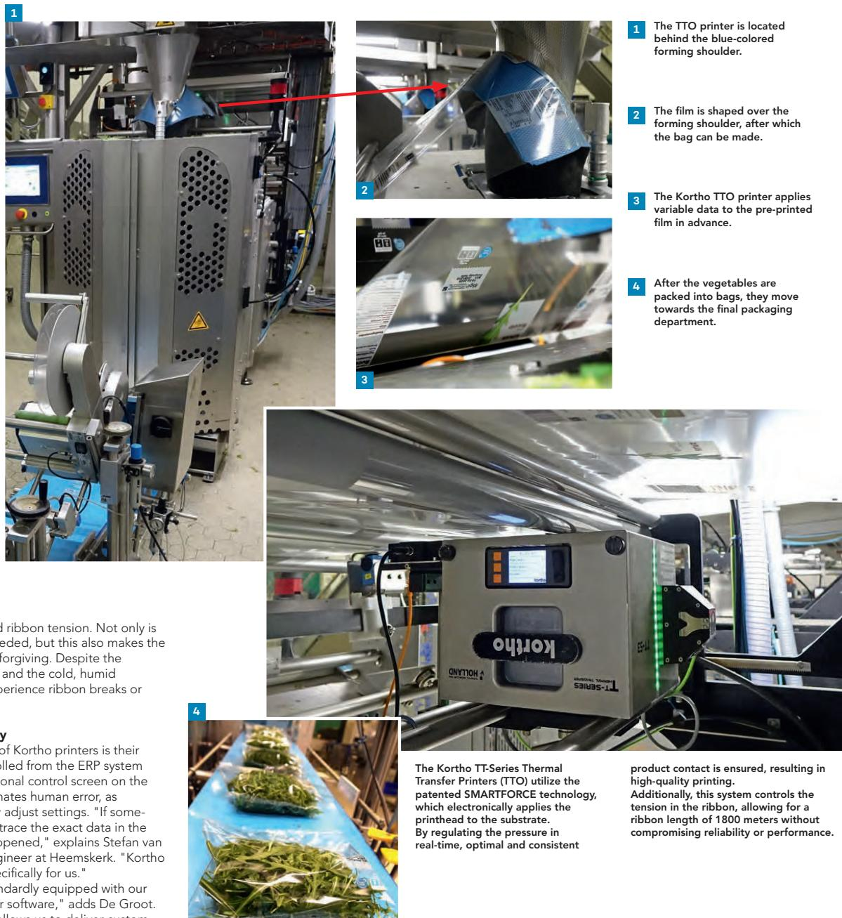
the printhead pressure and ribbon tension. Not only is pressured air no longer needed, but this also makes the printer highly reliable and forgiving. Despite the 1,800-meter ribbon length and the cold, humid environment, we never experience ribbon breaks or print quality issues."
